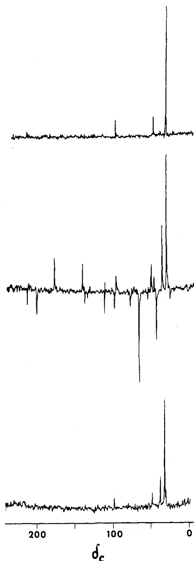
Figure 1. Proton decoupled carbon-13 FT NMR spectra of a 25% DTBK solution in \text{CCl}_4 obtained before (top), during (middle), and after (bottom) irradiation. The spectra width is 250 ppm. For each spectrum 100 free induction decays were accumulated at a pulse repetition time of 10 sec.
